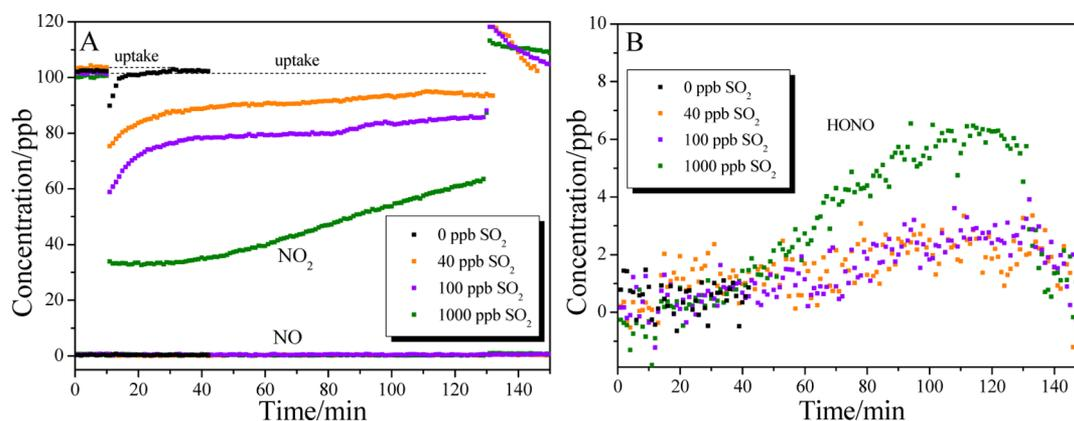
**Figure 1.** Comparison of NO<sub>2</sub> uptake on MgO in the presence of various SO<sub>2</sub> concentrations: 0 ppbv (177.42 mg, black), 40 ppbv (43.15 mg orange), 100 ppbv (33.47 mg, violet), and 1000 ppbv SO<sub>2</sub> (48.96 mg, olive). (A) NO<sub>2</sub> uptake and NO formation, (B) HONO formation. RH = 7.5%. Desorption of NO<sub>2</sub> occurred when the injector was pushed to the end of the flow tube after 120 min of reaction.
