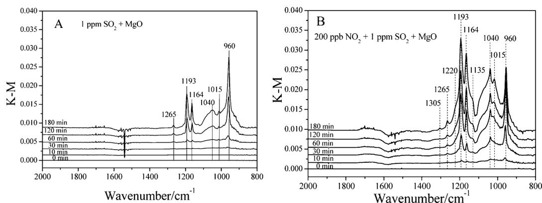
**Figure 5.** In situ DRIFTS spectra of MgO exposed to (A) 1000 ppbv  $\text{SO}_2$  and (B) 1000 ppbv  $\text{SO}_2$  and 200 ppbv  $\text{NO}_2$  as a function of time. RH = 4.5%.
