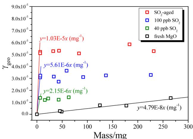
**Figure 2.** Mass dependence of initial geometric uptake coefficients ( $\gamma_{\text{geo}}$ ) of 100 ppbv  $\text{NO}_2$  on different MgO surfaces at 7.5% RH: fresh MgO (black),  $\text{SO}_2$ -aged MgO (red), and fresh MgO coexisting with 100 ppbv  $\text{SO}_2$  (blue) and 40 ppbv  $\text{SO}_2$  (olive).
