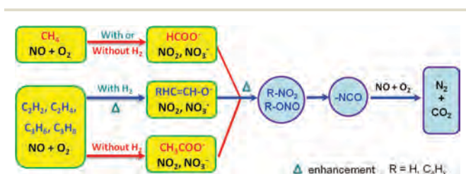
Fig. 6 Proposed mechanism of H 2 -assisted HC-SCR over Ag/Al 2 O 3 .
