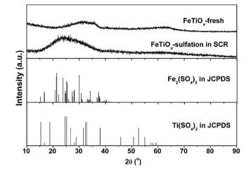
**Fig. 2.** XRD results of  $FeTiO_x$ -fresh and  $FeTiO_x$ -sulfation in SCR together with standard cards of  $Fe_2(SO_4)_3$  and  $Ti(SO_4)_2$  in JCPDS.
