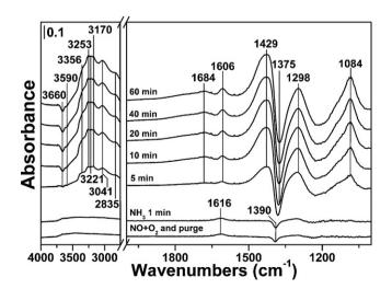
Fig. 7. In situ DRIFTS of reaction between  $NH_3$  and pre-adsorbed  $NO_x$  species at 200 °C over FeTiO<sub>x</sub>-sulfation.
