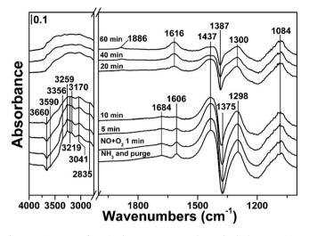
Fig. 8. In situ DRIFTS of reaction between NO +  $O_2$  and pre-adsorbed NH<sub>3</sub> species at 200 °C over FeTiO<sub>x</sub>-sulfation.
