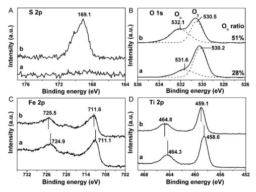
Fig. 4. XPS results of (A) S 2p, (B) O 1s, (C) Fe 2p and (D) Ti 2p in (a) FeTiO<sub>x</sub>-fresh and (b) FeTiO<sub>x</sub>-sulfation in SCR.
