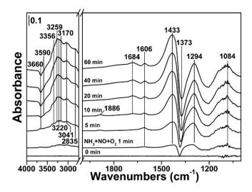
**Fig. 9.** In situ DRIFTS of reaction in NH<sub>3</sub> + NO + O<sub>2</sub> at 200 °C over FeTiO<sub>x</sub>-sulfation.
