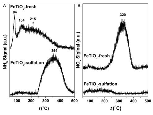
Fig. 6. (A) NH<sub>3</sub>-TPD and (B) NO<sub>x</sub>-TPD over FeTiO<sub>x</sub>-fresh and FeTiO<sub>x</sub>-sulfation.
