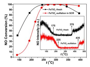
**Fig. 1.** SCR activity over  $FeTiO_x$  catalysts before and after sulfation (inset: TPSR in a flow of  $NH_3 + NO + O_2$ ).
