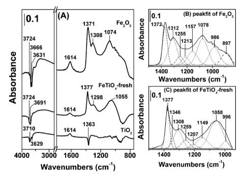
Fig. 5. In situ DRIFTS of SO<sub>2</sub> + O<sub>2</sub> treatment on Fe<sub>2</sub>O<sub>3</sub>, FeTiO<sub>x</sub>-fresh and TiO<sub>2</sub> at 200 °C for 2 h and then N<sub>2</sub> purge for 0.5 h.
